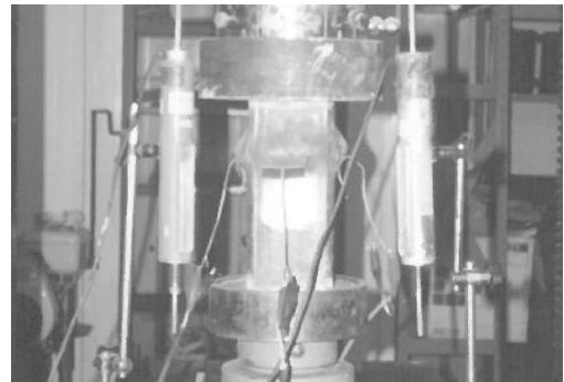
Fig. 7. Local buckling of a concrete-filled steel tube
