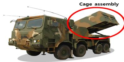
Fig. 2. Cage assembly of K-MLRS Launcher
