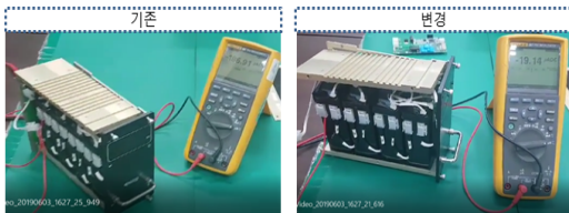
Fig. 22. Measured result of leakage current about Improved point in control board
