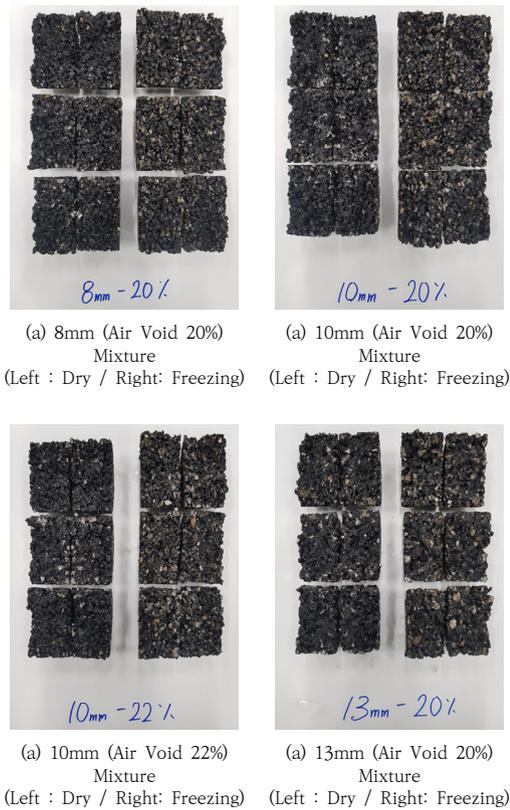
Fig. 3. Specimen Splitted after Indirect Tensile Strength Test
