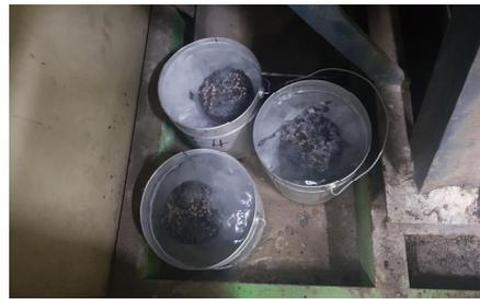
(a) Specimen Freezing at  $-18^{\circ}\text{C}$  for 16hours
