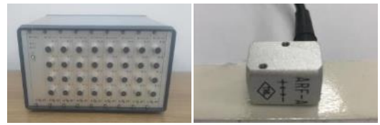
(a) Data Logger (b) Accelerometer
