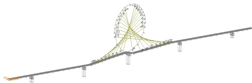
(b) B Bridge Cable Analysis Tension
