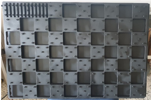
Fig. 5. Thermal checkerboard used for calibration
