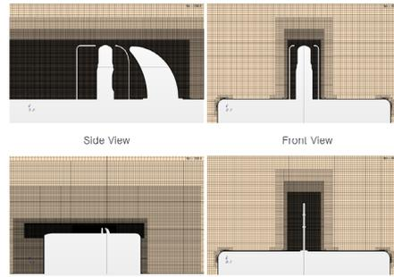
Fig. 9. Computational mesh for head cover with protector
