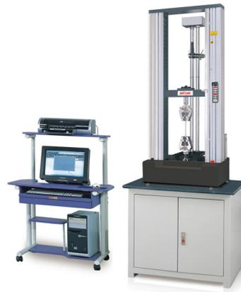
Fig. 4. Universal testing machine
