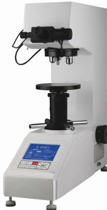
Fig. 3. Vickers hardness tester
