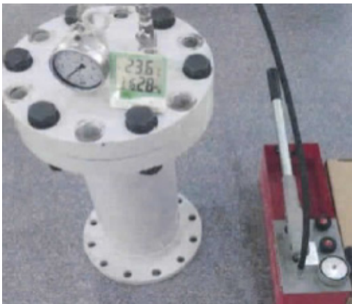
Fig. 9. Pressure chamber and test pump
