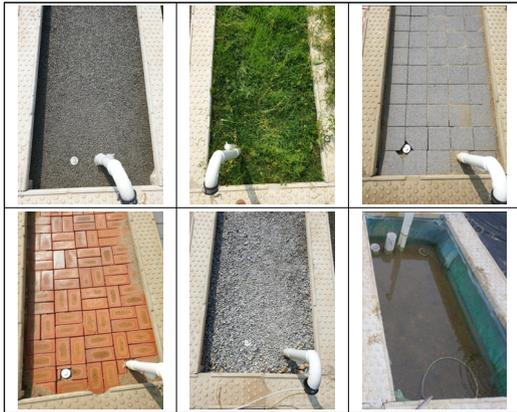
Fig. 2. Classification of experiments according 6 ground materials
