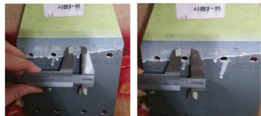
Fig. 14. #2-24 g Liquid Penetrant Inspection
