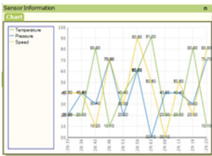
Fig. 5. An example of displaying piping status trend over time for values measured from IoT sensors
