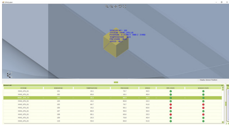
Fig. 4. An display example of operation status and measured value of IoT sensors on the grid view
