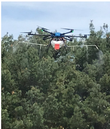
Fig. 8. Field performance evaluation of water fog spraying system using drone(EFT-E610)
