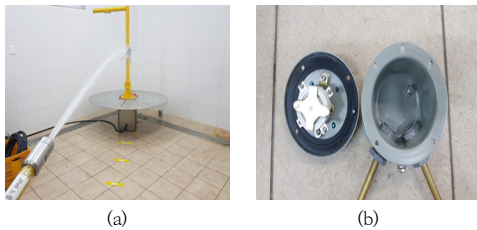
Fig. 13. Ingress protection test (a) Under testing (b) Check inside of enclosure
