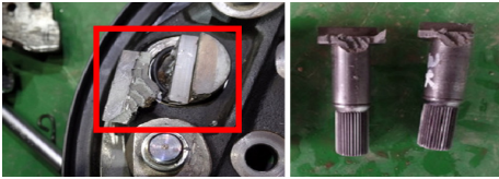
Fig. 2. Shape of broken cam on parking brake drum
