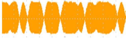
Fig. 8. Designed PSK31 output waveform
