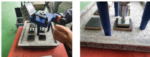
Fig. 5. Adhesion strength
