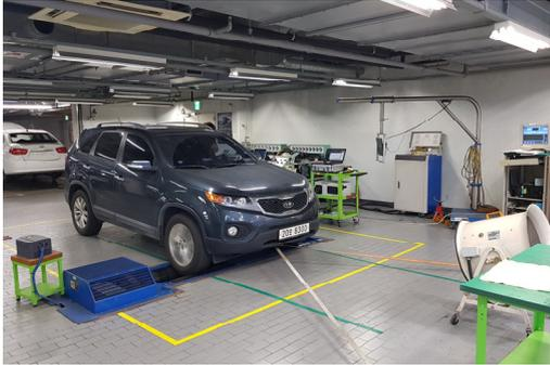
Fig. 1. View of emission test of test vehicle driving with kd-147 mode
