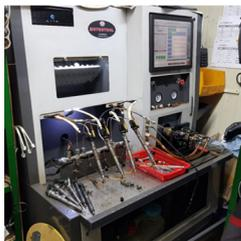
Fig. 2. Injector tester
