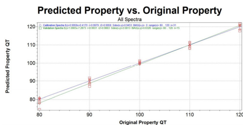
Fig. 4. NIR original spectra linearity test
