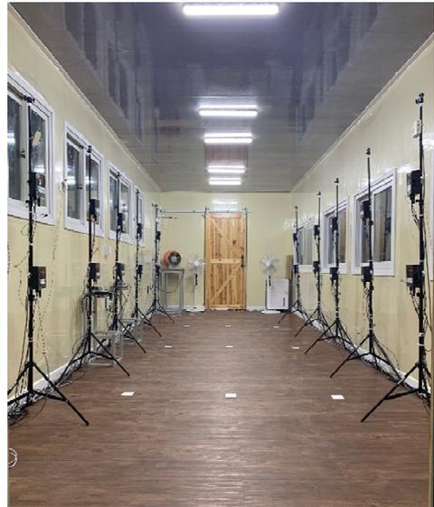
Fig. 1. Inside the simulation chamber for particulate matter suspension experiments.
