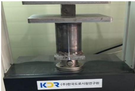
Fig. 3. Compressive Strength Test for the Specimen
