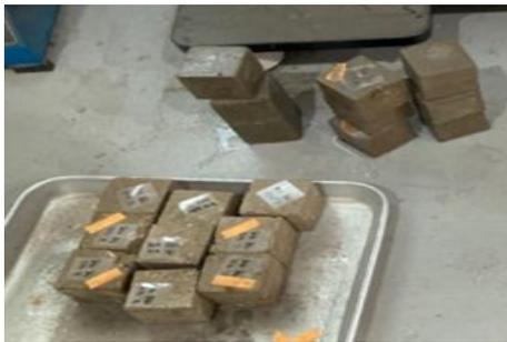
Fig. 2. Cubic Molds for Compressive Strength Test
