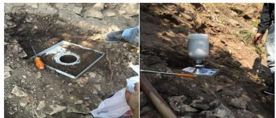
Fig. 3. Field Density Test[22]
