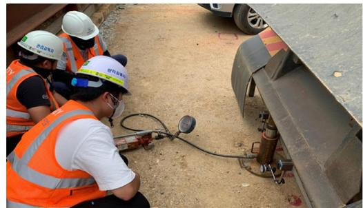
Fig. 2. Plate Bearing Test
