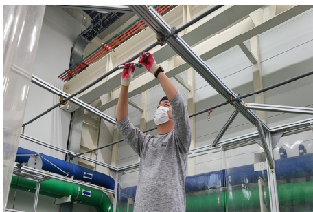
Fig. 7. Replacing the Nozzle to Change the Rainfall Intensity
