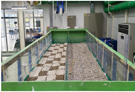
Fig. 5. Outflow Test Set with Porous Area - 33%
