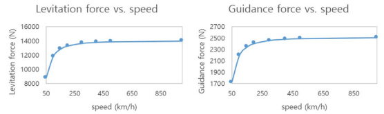
Fig. 7. Levitation and guidance force according to speed (at \Delta z, \Delta y=30 mm)
