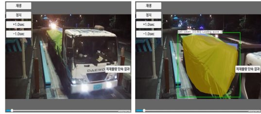
Fig. 9. Recognition result of the vehicle enforcement system for bad loading
