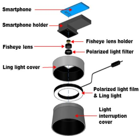
Fig. 2. Exploded view of image acquisition system for beef carcass grading
