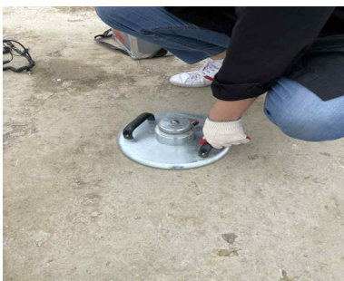
Fig. 8. Placement of Loading Plate on the Solidified Soil Base
