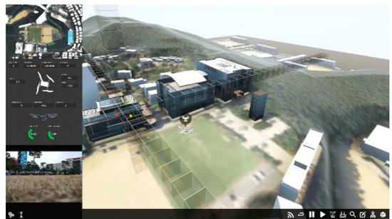
Fig. 12. Layout for virtual reality based UAV monitoring and auto-flight route providing system
