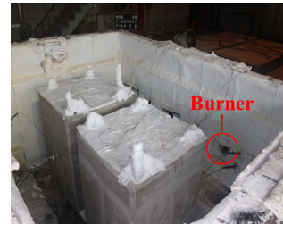
Fig. 4. Fire test set-up of specimen
