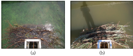
Fig. 3. Plan view of debris accumulation test (a) Woody plants, (b) Herbal+woody plants
