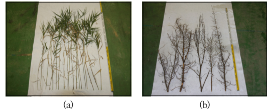
Fig. 2. Debris sample for accumulation experiments (a) Herbal plants, (b) Woody plants
