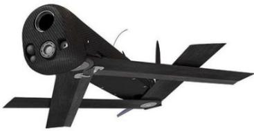
Fig. 2. Switch blade 300 - Aero Vironment(USA)
