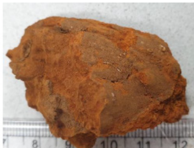
Fig. 5. Field collected corrosion sample
