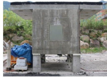
Fig. 4. 150mm bridge specimen (Box D)
