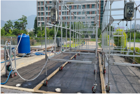
Fig. 6. Simulator of artificial rainfalls for porous pavement
