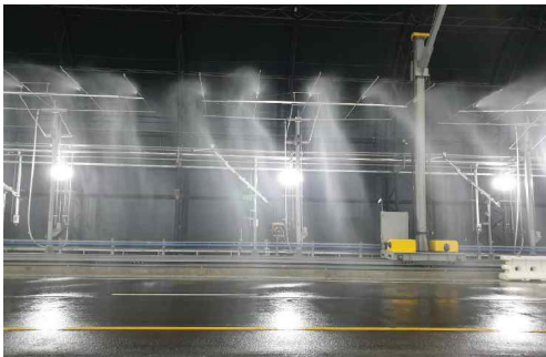
Fig. 3. Rainfall weather conditions in the test section
