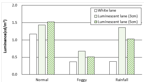
Fig. 7. Luminance measurement results by weather conditions with headlight
