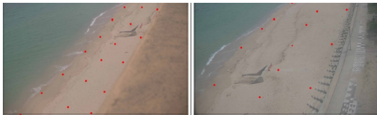
Fig. 3. Calibration of monitoring image at reference point for wave runoff analysis
