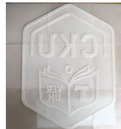
Fig. 9. Disposable form liner printed by 3D printer
