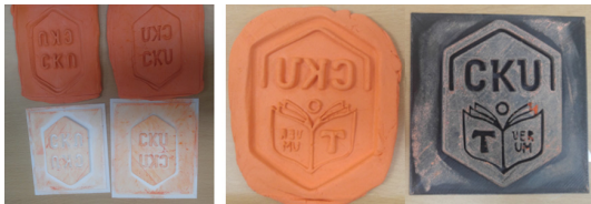
Fig. 3. Confirmation of shape production and applicability test using clay
