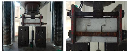
Fig. 6. Shear test for three layers of bricks
