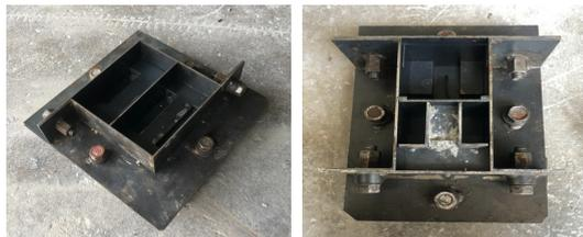
Fig. 3. Steel mold for interlocking concrete bricks
