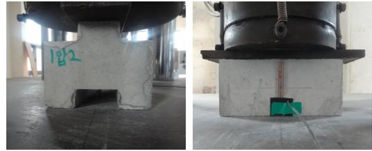
Fig. 4. Compression test of middle type brick
