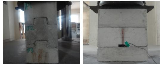
Fig. 5. Prism test for three layers of bricks
