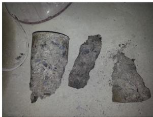
(a) Failure Shape of Specimen
