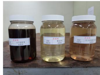
Fig. 7. Admixtures used in the Experiment (Naphthalene Series, Inorganic A(Melamine Series) and Inorganic B from Left Side)
