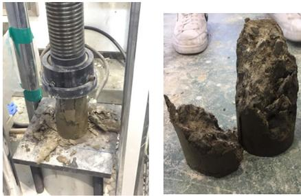
(a) compressive shape (b) failure shape
