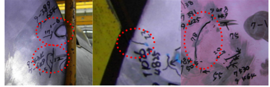
Fig. 1. Visual inspection results of cracks on surface of the propeller
