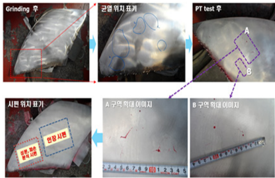
Fig. 3. Check blade crack point and mark specimen position
