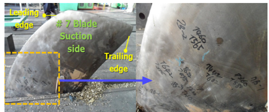
Fig. 2. Propeller blade cutting for specimen
