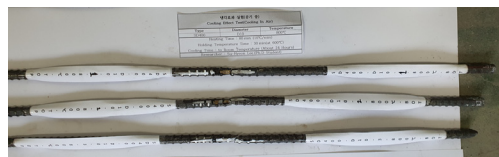
Fig. 18. Test results of SD400 D10 800 °C in cooling in air(CIA) test
