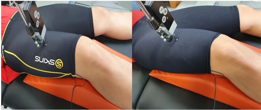
Fig. 2. Example of measuring lower extremity muscle contraction by compression garment fabrics. Left: control (skins, nylon 75% + spandex 25%); Right: type A (polyester 77% + spandex 23%).
