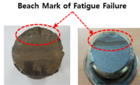
Fig. 4. Fatigue failure section of HSU Bolt
