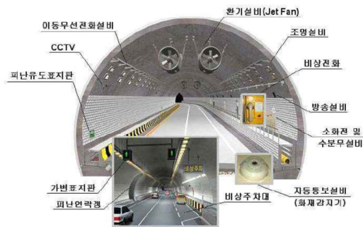
Fig. 2. Disaster prevention facilities in tunnel[21]
