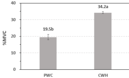
Fig. 11. Total %MVC by weeding methods.(PWC : Prototype Weeding Cultivator, CWH : Conventional Weeding by Human)
