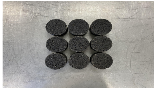
Fig. 7. Specimens of FNS Asphalt Concrete
