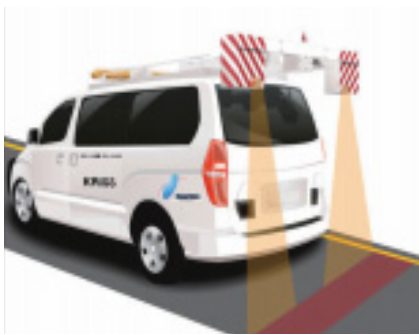
Fig. 2. Road pavement survey vehicle equipped with 3D laser scanning camera
