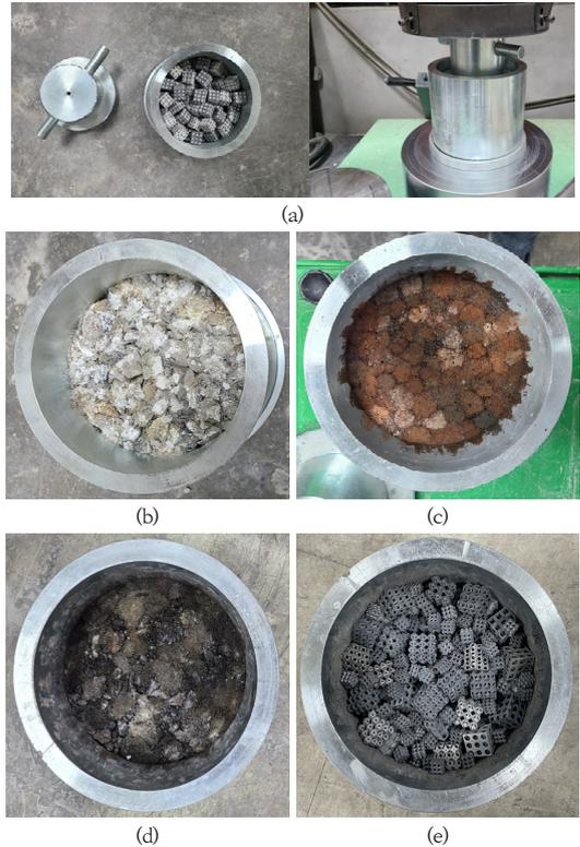
Fig. 4. Situation after aggregate crushing test
