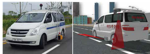
Fig. 2. Vehicle-mounted lane painting luminance and quality inspection device.
