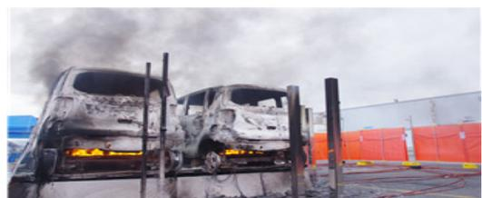
Fig. 12. Instant photographs during the fire in the battery
